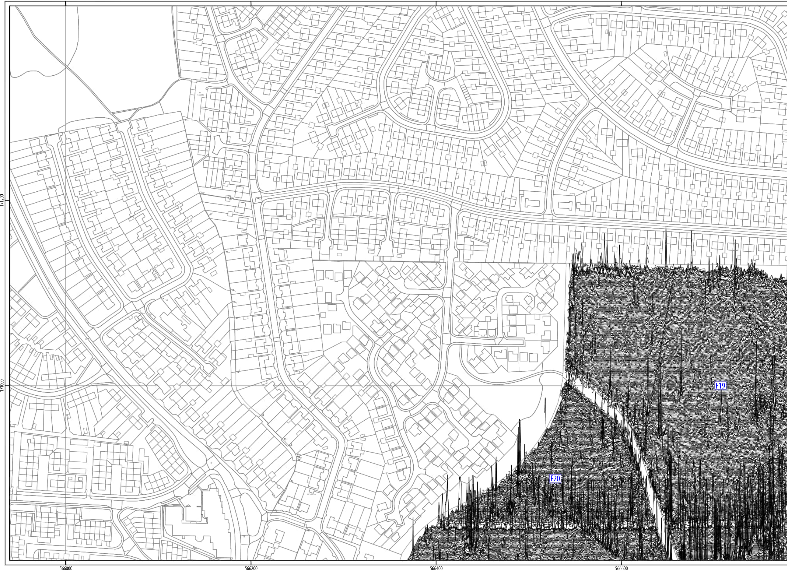
ILLUS 28 XY traceplot of minimally processed magnetometer data; Sector 6
